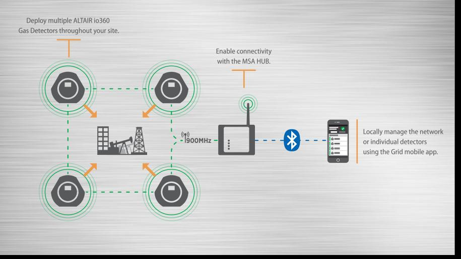
Each MSA HUB can support up to 32 ALTAIR io360 Gas Detectors. The 868 MHz HUB (select countries in Europe, Africa, and Middle East) supports up to 16 detectors.
