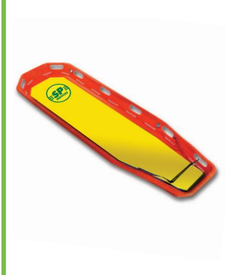
The Basket Stretcher is a rigid stretcher with multiple handholds & lifting points as well as a foot plate, designed for hand, rope or helicopter rescue. The newly designed shell makes this stretcher ideal for a wide range of rescue situations. The shell is built from high density cross linked polyethylene which is resistant to splintering and cracking. The surface is impervious to body fluids and petroleum products making it easy to keep clean.
