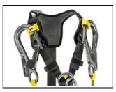
The MGO connectors on fall arrest lanyards can be stowed on each shoulder strap. The user is thus unhindered by the lanyard, and the connectors stay within reach. In case of a fall, the system releases the MGOs and allows the absorber to be deployed.
