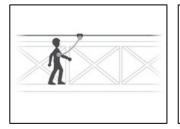
ABSORBICA-I single lanyards are designed particularly for protection on a horizontal lifeline or on an elevated platform.
