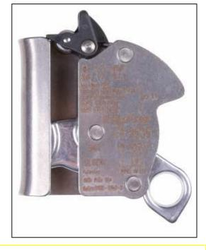
Designed to provide vertical/inclined fall protection to operatives ascending /descending a ladder or structure, and is for use with 11mm Kernmantel Rope Only. When used by itself, it should be connected directly to the chest attachment of a compatible harness via a karabiner. This ensures that the user is held close to the structure and, in the event of a slip, the fall distance and loading on the top anchor is minimal.
