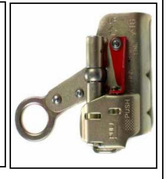
The RGA10 is designed to provide vertical/inclined fall protection to operatives ascending /descending a ladder or structure. This version of the rope grab is for use with **16mm Hawser Laid Rope Only**. This unit comes standard with a shock pack fitted and cannot be removed, however due to the "gate opening" method of attachment, the RGA10 offers positive closure and good camming action. The locking cam on this device is toothed and arrests well on the hawser laid rope.
